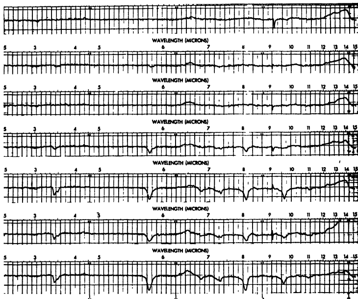
FIG. 1. Infrared patterns of components separated from commercial solvents by gas chromatography.
